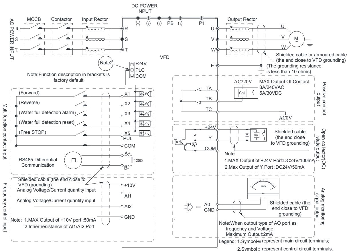
Note: When connect solar panel, both AC input (R, T) and DC input (+, -) is okay, AC input is prefer.
